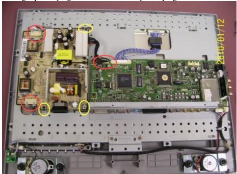
backlight power plugs and the black CPU power plug as shown circled in Red.
