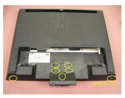
The case will pop open if you insert a small flat screwdriver between the 2 halves and apply a gentle pressure. Once it starts opening just use your fingers and work your way around the screen.
