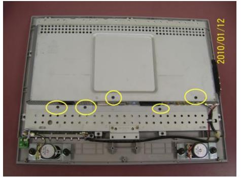
With the shield off we can now see the board that we will be working on. Remove the 3 screws holding the power supply board in place they are circled in Yellow. Next disconnect the 2
