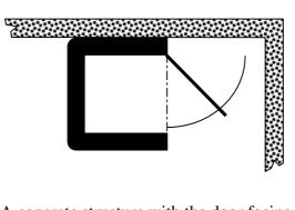
A concrete structure with the door facing a concrete wall will act as a perfectly serviceable nuclear storage safe. A steel filing cabinet is easily encased in this manner, allowing easy access to the materials inside.
