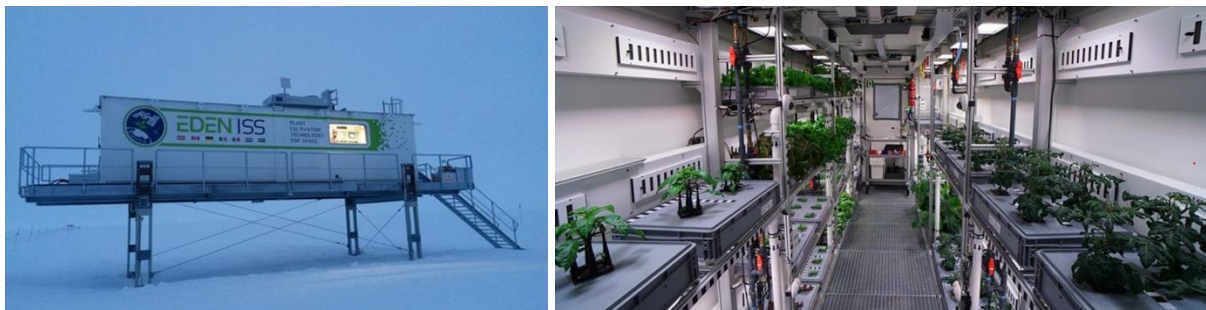
Figure 3.1: EDEN ISS Mobile Test Facility (left: outside view; right: inside view of cultivation area just after seeding) [6]
