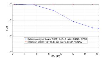
Figure 13. FER in AWGN, simplified MUD. Bearer F80T1Q4B-L8 (QPSK rate 1/3, symbol rate 33600 sym/sec, roll-off 0.25) is used for the reference signal while bearer F80T1X4B-L3 (16 QAM rate 1/3, symbol rate 33600 symbols per second, roll-off 0.25) is used for the interferers. Note that rate 1/3 is the lowest code rate available in [10]). The interference pattern for beam 110 EoB detailed in Table I (worst case scenario) has been used.
