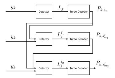
Figure 3. Block diagram illustrating an iteration of the SISO detector/decoder.
