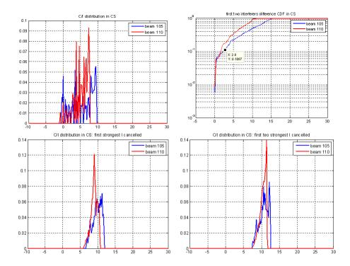
Figure 8. Distribution of interference across the covered area in case: 1) all interferers are present (topleft), 2) the strongest interferer has been removed (bottom-left), 3) the two strongest interferers have been removed (bottom-right). The CDF of the difference between the two strongest interferers across the beam is also shown (top-right).
