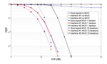
Figure 4. FER curves for the reference signal and for two interferers. The interferers have a relative C/I of 0 and 6 dB, for a global C/I of -0.9732 dB. A bearer with QPSK modulation, rate 1/3 and 360 data bits per FEC codeword have been used for all signals.
