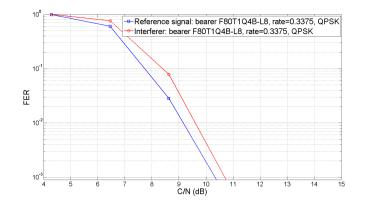
Figure 11. FER in AWGN, simplified MUD. Bearer F80T1Q4B-L8 (QPSK rate 1/3, symbol rate 33600 sym/sec, roll-off 0.25) is used for all signals. The interference pattern for beam 110 EoB detailed in Table I (worst case scenario) has been used.
