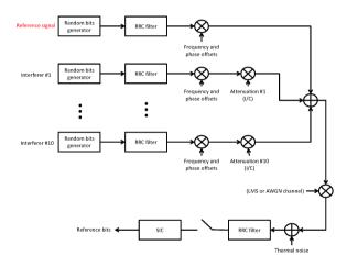
Figure 10. Simulation setup in AWGN and LMS channels.
