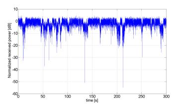
Figure 14. Five minutes sample of the 30 minutes channel series (power in logarithmic scale) used in the simulations. The time series has been generated with a channel simulator implementing the LMS Perez-Fontan model in suburban environment, vehicle speed 50 kmph and satellite elevation 30°.
