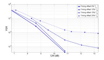
Figure 16. FER in AWGN, simplified MUD, QPSK rate 1/3 used in all signals. Curves for different relative delays are shown. Delays are expressed in fraction of symbol duration  $T_s$ .
