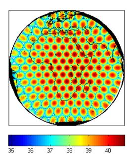
Figure 2. Antenna beam pattern gain [dBi].
