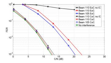
Figure 15. Frame error rate for the reference signal using the simplified SIC scheme with one iteration (one detection and one decoding iteration). A 30 minutes LMS channel series in suburban environment generated according to [23] has been used. 10 interferers have been considered using the C/I values in Table I. Bearer F80T025Q1B-L8 (QPSK, channel code rate 1/3, symbol rate 8400 symbols per second) of standard [10] has been adopted for all signals.
