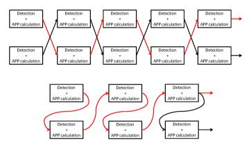
Figure 6. Comparison between the proposed method and a parallel MUD scheme. In red we put into evidence the decoding path for the reference signal. In the figure we show only the propagation of the APPs. In the practical implementation of both schemes the detector takes as input also the received signal, not indicated for sake of clarity.
