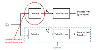
Figure 9. Proposed simplified SIC scheme. Only the strongest interferer is taken into account and no iterative detection/decoding is applied (i.e., reference signal is detected as described in Section 3 and decoded using the turbo decoder specified in [10]). Optionally, also the strongest interfering signal can be decoded.
