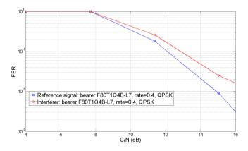
Figure 12. FER in AWGN, simplified MUD. Bearer F80T1Q4B-L7 (QPSK rate 2/5, symbol rate 33600 sym/sec, roll-off 0.25) is used for all signals. The interference pattern for beam 110 EoB detailed in Table I (worst case scenario) has been used.
