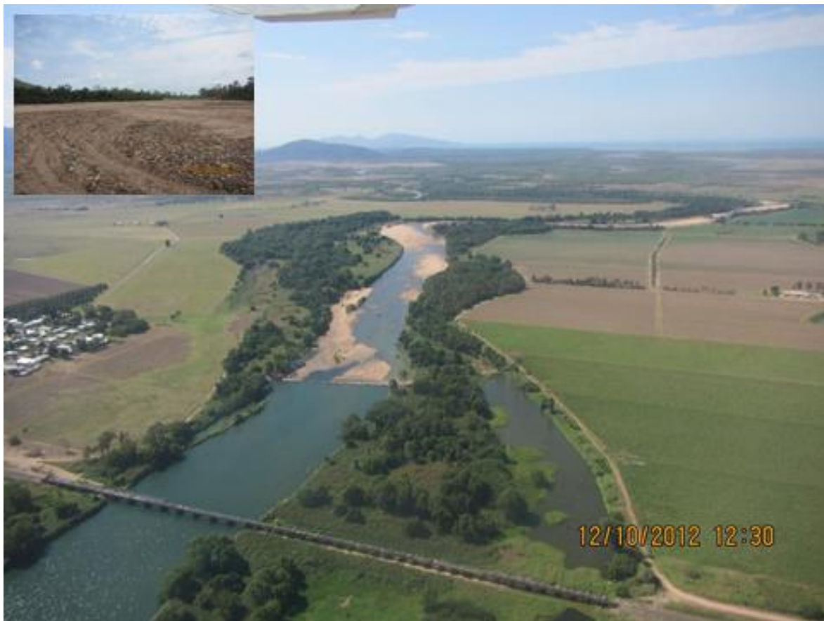
Figure 2.4.2: Weirs and erosion from grazing of natural areas is causing the Haughton River to fill with sand, both above (inset) and below the weirs (main picture). The weir traps heavier sediments above the weir and the reduced water velocity below the weir fails to move the coarser sand to the coastline. Interestingly the beach at the coastal settlement of Cungulla is eroding
