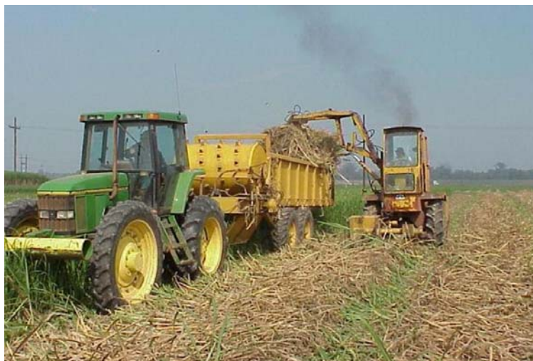
Field loader (at the back) collects cane from heap row and transfers it to the planting wagon
