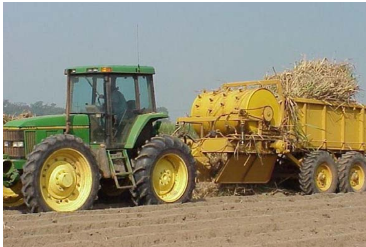
Mechanical planter (drum planter) plants one row at a time
