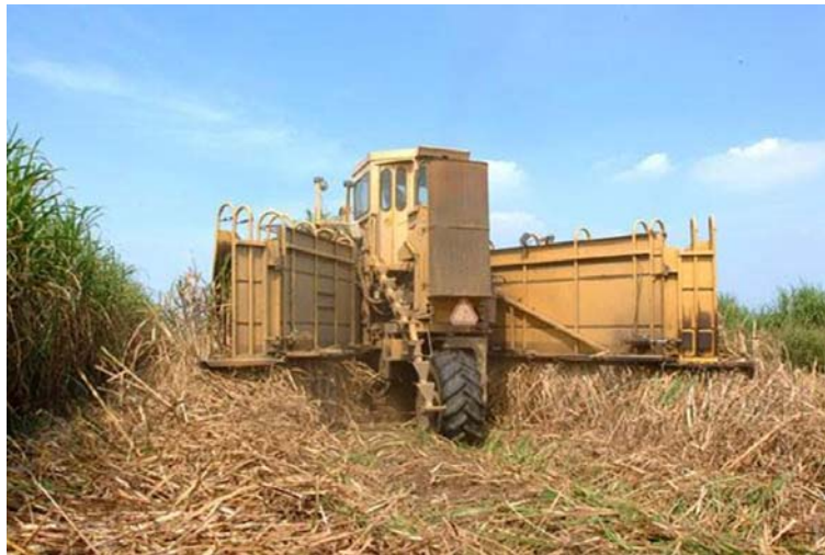
Soldier harvester in action – two rows at a time, resulting in two heap rows behind
