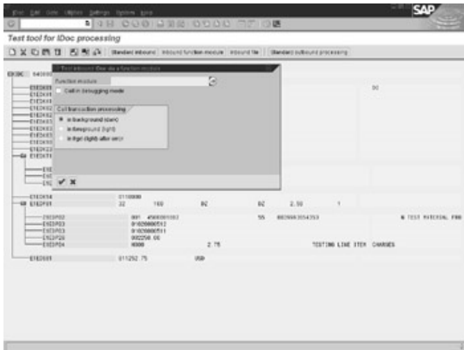
Figure 10.10: The dialog box for testing an inbound IDoc via a function module (© SAP AG)
