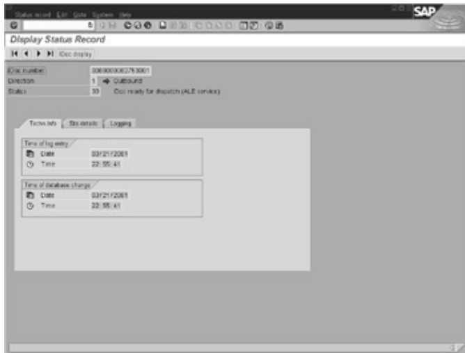
Figure 30.14: Details of a status record as viewed using the IDoc display tool (© SAP AG) Status records have the following characteristics.
