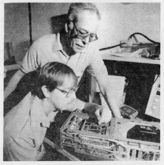
Ray Ochoa and Terry Hurst (seated) setting calibration on the heading servo in the Flight Data Recorder.
