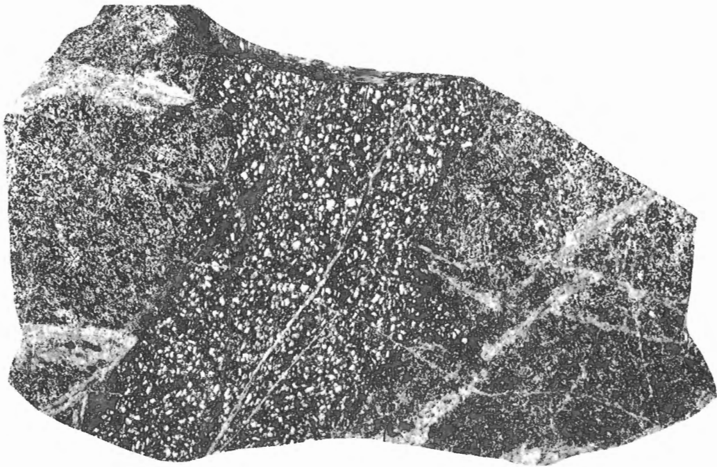
Figure 18. 17.a Porphyry Copper, Molybdenum, Tungsten. Granisle mine, British Columbia. Intermineral porphyry dyke cuts fine grained porphyry, magnetite- and chalcopyrite-bearing quartz veins, and is cut by chalcopyrite-bearing quartz veins. Sample is 25 cm long. Sample: R.V. Kirkham (GSC 201531-M).
