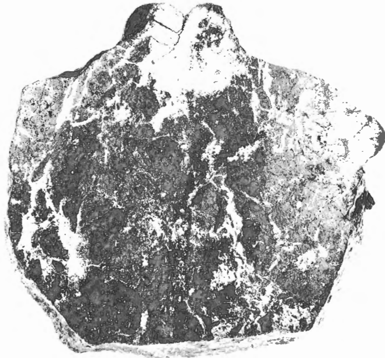
Figure 19. 17.b Porphyry Copper, Molybdenum, Tungsten. Pit No. 2, Copper Mountain, British Columbia. Typical erratic, discontinuous veins, lenses, and disseminations of chalcopyrite (white) in intensely altered monzonite. Sample is 17 cm high. Sample: R.V. Kirkham (GSC 203886-G).
