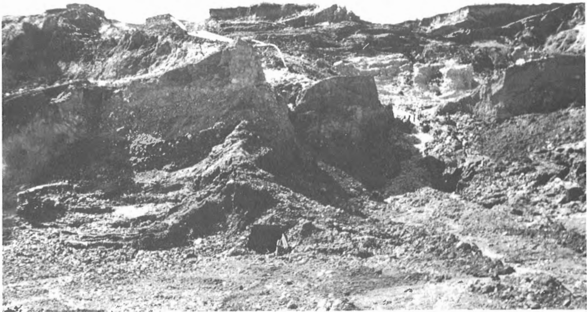
Figure 6. 5.2 Placer Gold. Klondike area, Yukon. Basal part of high level White Channel bench gravels. Early placer miners (c.1902) followed lower bedrock surface with timbered drift (about 1.2 m wide). Bench mined hydraulically and with bulldozer in 1960. Photo: C.R. McLeod (GSC 202282-V).
