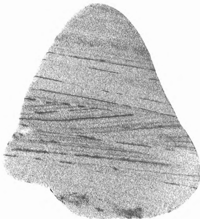
Figure 8. 6.2 Sandstone Lead. Yava deposit, Nova Scotia. Galena and carbonaceous material (mainly wood trash) oriented parallel to bedding in crossbedded terrigenous sandstone. Wood trash is detrital; galena occurs as cement between quartz grains. Sample is approximately 20 cm high. Sample: R.V. Kirkham (GSC 203641-S).
