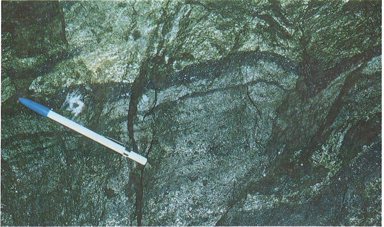
Plate 6. 9.1 Volcanic-Associated Massive Sulphide. Lake Dufault mine, Noranda, Quebec. Typical well bedded, massive ore: pyrite (dull brassy yellow), chalcopyrite (bright yellow), sphalerite (dark metallic blue-grey). Photo: R.V. Kirkham.
