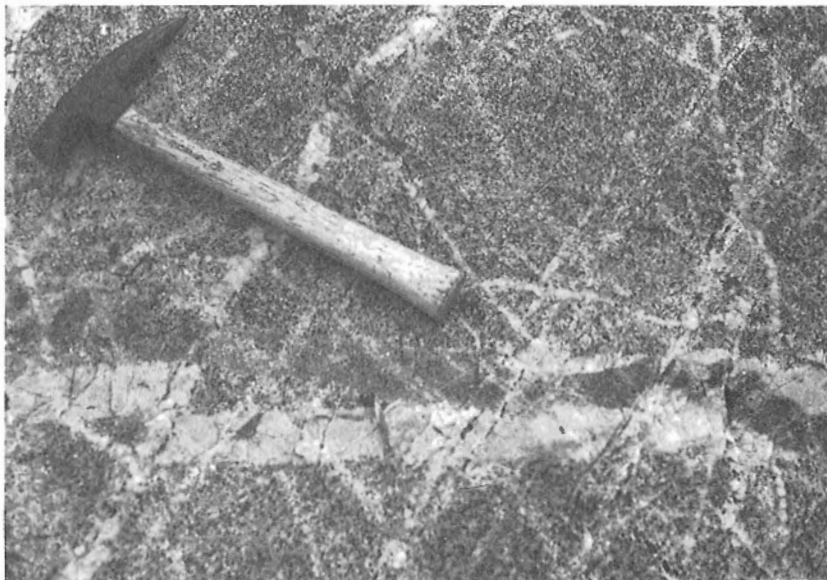
Figure 21. 17.c Porphyry Copper, Molybdenum, Tungsten. Kitsault mine, British Columbia. Typical molybdenite-bearing quartz vein stockwork cutting porphyritic granodiorite and aplite dykelet. Photo: R.V. Kirkham (GSC 3-16-72).
