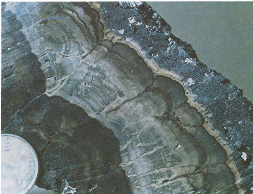
Plate 2. 6.1 Mississippi Valley Lead-Zinc. Pine Point, Northwest Territories. Typical botryoidal textured sulphides. Layered sphalerite (dark brown and white) overlain by coarse grained galena (steel blue). Sulphides precipitated in cavity beginning at lower left, with successive layers added into open space to right; last sulphide deposited was galena. Photo: D.F. Sangster.
