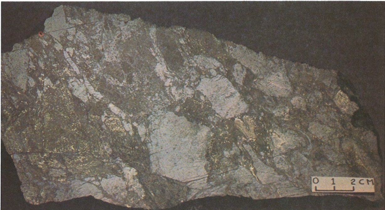
Plate 8. 9.1 Volcanic-Associated Massive Sulphide. York Harbour deposit, Newfoundland. Typical fragmental massive sphalerite (grey)-chalcopyrite-pyrite ore. Note contorted, well laminated chalcopyrite clast. Photo: R.V. Kirkham.
