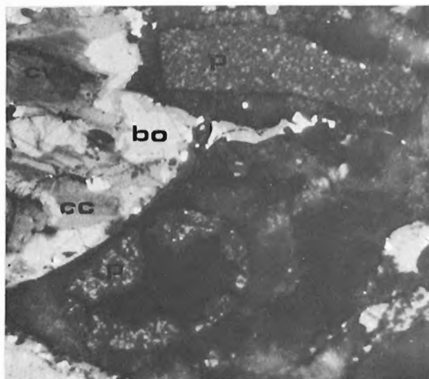
Figure 60.1. Photomicrograph (reflected light, air, X1000) Pitchblende(?), grey(p) with numerous sulphide inclusions. Light area is bornite (bo) surrounded by chalcocite(cc) and covellite(cv); galena (white) occurs as small crystals throughout the sample. The undefined matrix is mainly calcium carbonate.
