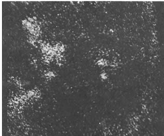
Figure 60.4. Distribution of iron. Fe K \alpha X-ray picture of area covered in Figure 60.1 (X1000).
