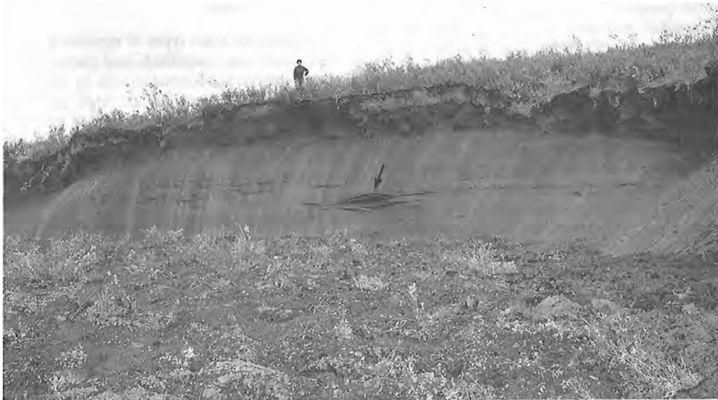
Figure 6. A clay pod (marked by an arrow), in massive segregated ice to the southeast of Tuktoyaktuk; note person for scale.
