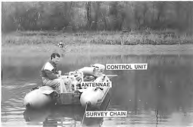
Figure 2. Profiling channel bottom sediments from an inflatable boat.
