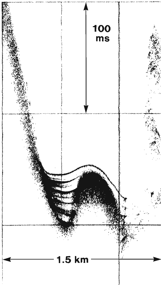
Figure 3. Cross-channel 3.5 kHz profile 43 in Knight Inlet, showing a structureless area within the sediments due to gas bubbles, and diffuse reflections at either end from the crystalline bedrock sides of the fiord.
