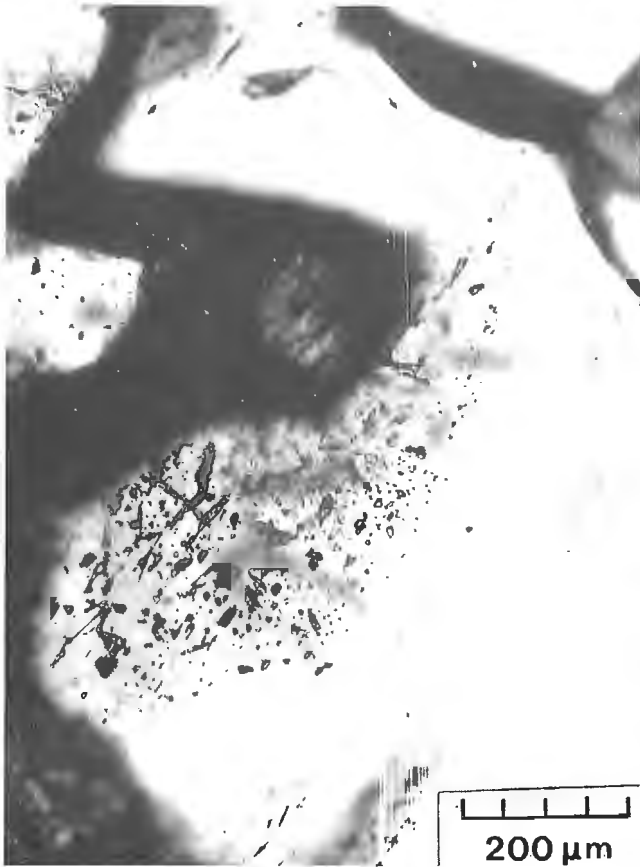
Figure 4a. Photomicrograph of cluster of primary fluid inclusions confined to growth zone defined by yellow sphalearite adjacent to inclusion-free white sphalearite.
