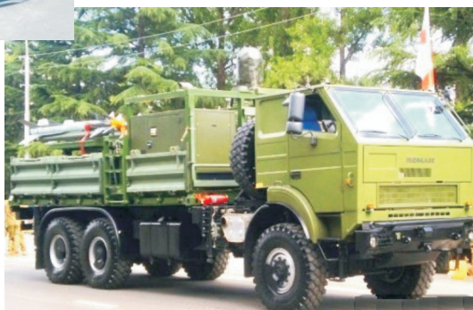
The SPIDER System used by Georgia is mounted on a ROMAN chassis and uses the PYTHON-5 Missile 16
