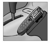
When installing the fixed mobile car phone avoid positioning the transceiver unit where it may disrupt the proper operation of the vehicle and/or its components, such as car stereo, air bags, cubbyhole, glove compartment, ashtray, lighter, gear stick,
