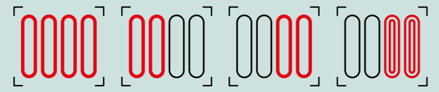
BOTH ZONES 3,000 WATT LEFT ZONE 1,500 WATT RIGHT ZONE 1,500 WATT TURBO ZONE 3,000 WATT
