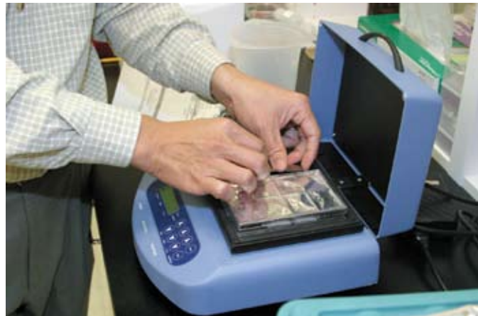
Chamber being placed into a ThermoShaker, which can process up to 32 arrays in one day.
