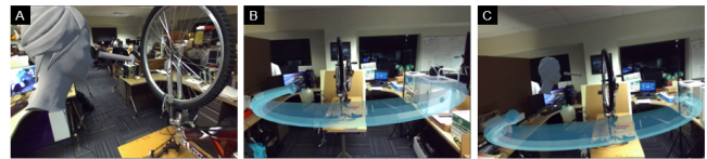
Figure 9: (A) A Virtual head indicating direction and position of where the next instruction will begin; (B) a navigational arrow rendered on the AR work space, based on the authors' movement; (C) the adaptive POV trigger and navigational arrows can be used together.
