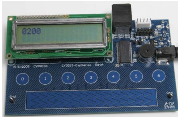
Figure 14. CY3213—CapSense Training Evaluation Board
