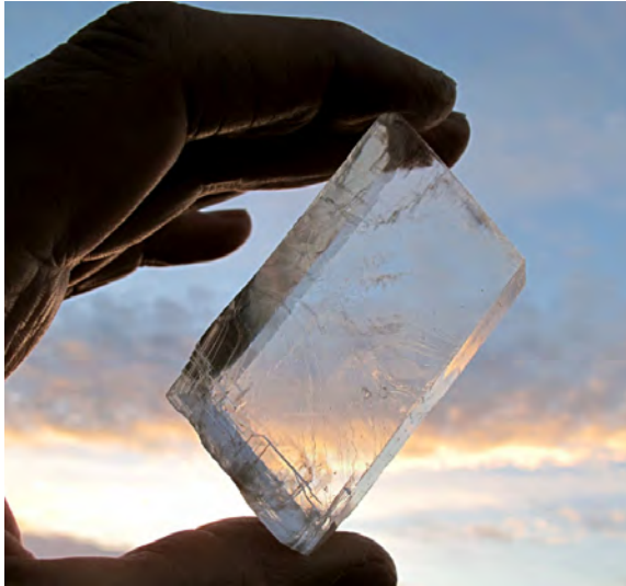
Figure 34.3: A sunstone can indicate the polarization of the scattered light. From that, one can deduce where the sun is located (courtesy of Wikipedia).
