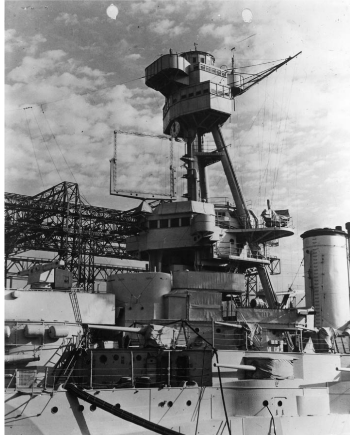
Photo # NH 77350 Prototype XAF radar antenna on USS New York
