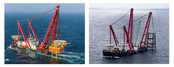
*Figure 6-17 Examples on transport of Topside and Jacket in crane hook.*
