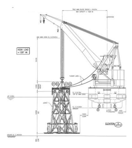
*Figure 6-14 Lifting and jacket (example).*
