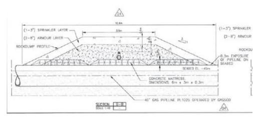
*Figure* 6-9 *Cross section of the crossing between the Europipe I and the pipeline bundle.*
