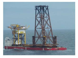
*Figure 6-18 Example of transport on barge.*
