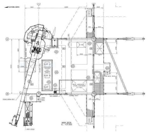
Figure 6-4 Keyplan of the topside main deck level.
