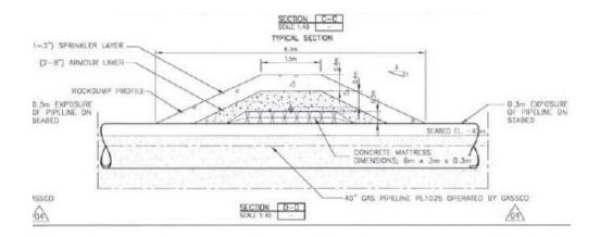
*Figure 6-10* Cross section of the crossing between the Europipe I and the umbilical.
