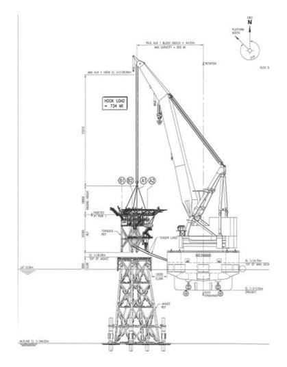
Figure 6-12 Lifting of Topside (example).
