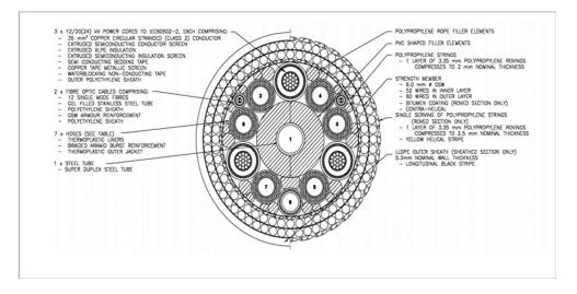
*Figure 6-11 Cross section through the umbilical.*
