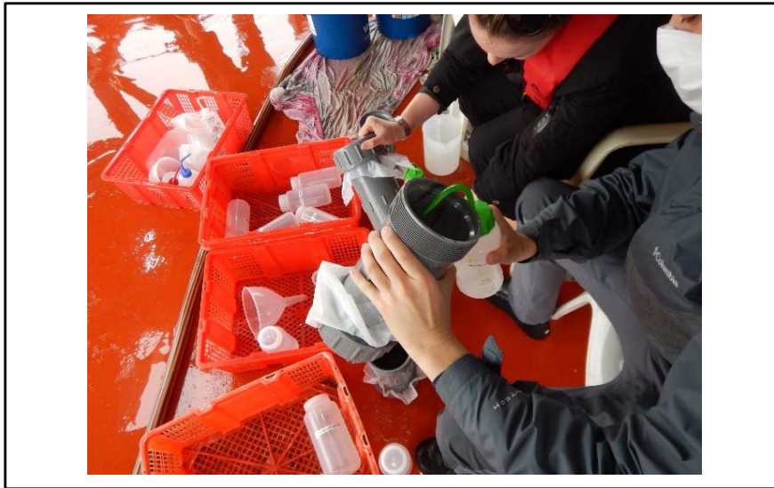
c) Seawater sample was filtered immediately using 10 \mu m mesh to collect the phytoplankton samples.
