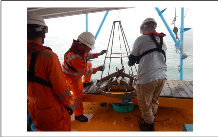
a) Sediment samples were collected using a modified Van Veen grab sampler.
