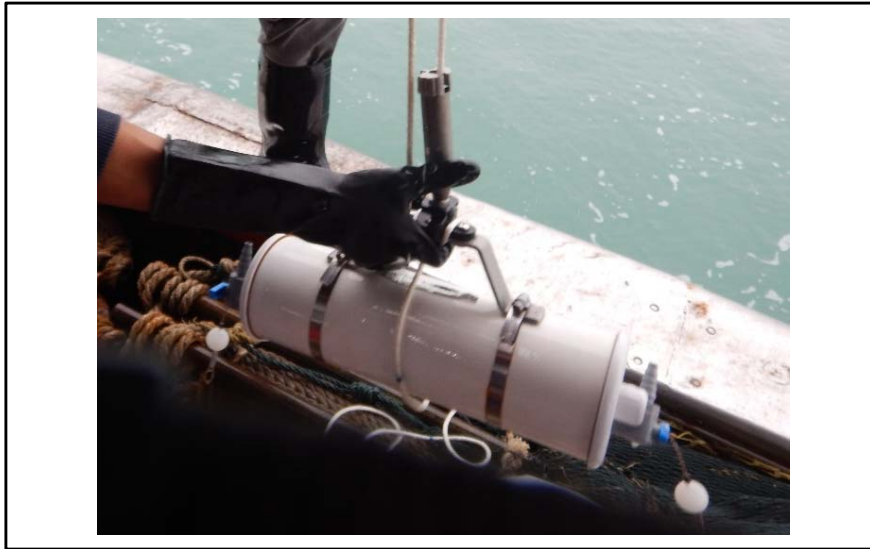
a) A Van Dorn Bottle Sampler was used to collect seawater sample.
