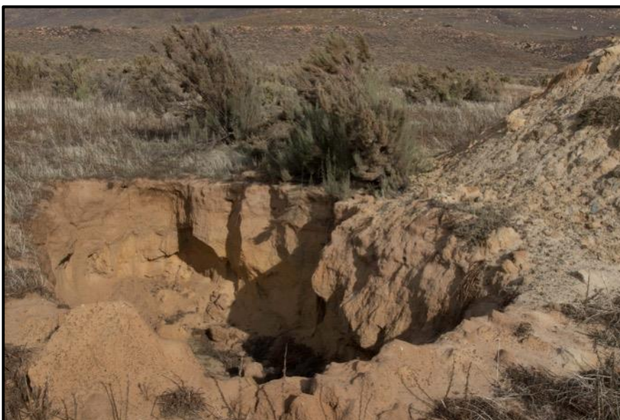
Figure 26. A soil pit in the alluvial sandy soil of the proposed Toeka Dam site.
