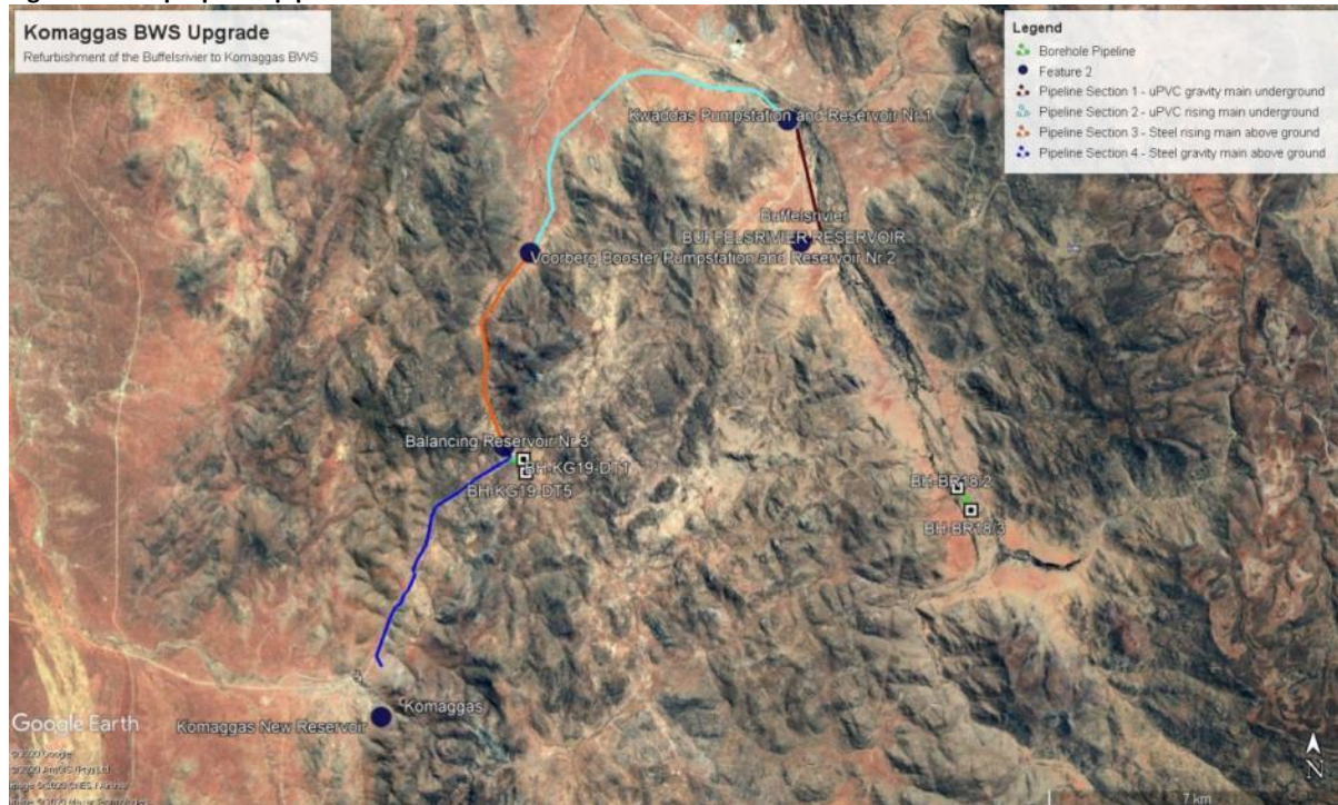
Figure 2: The proposed pipeline route and reservoir sites.
