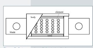
Figure 3: Cut away view of short circuit element
