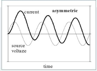
Figure 2: Typical short circuit current waveform
