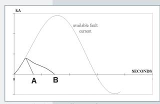
Figure 5: Clearing time effects on I<sup>2</sup>t
