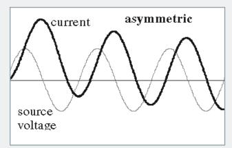
Figure 6: Asymmetrical current waveform
