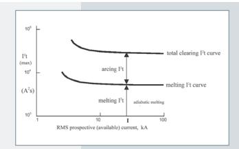
Figure 8: I<sup>2</sup>t versus available fault current
