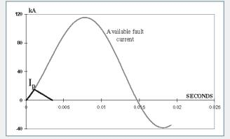
Figure 4: Current Limited Waveform
