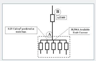
Figure 1: One-line diagram
