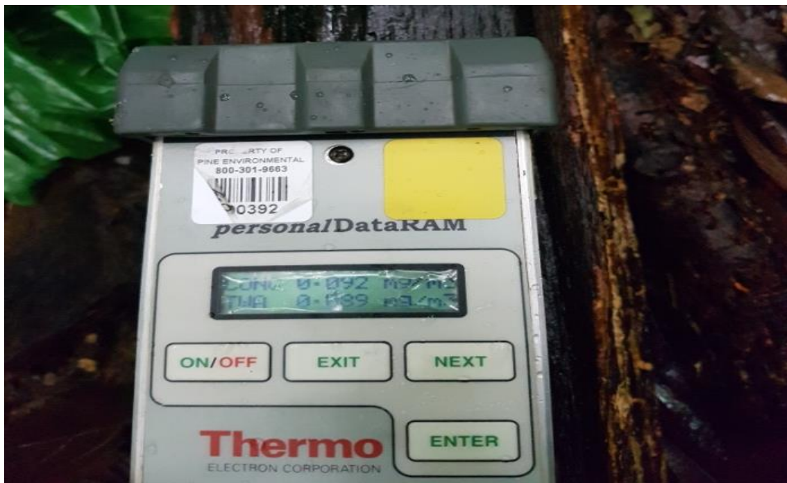
Figure 26: Photograph of the Thermo pDR-1000AN personal DataRAMTM Particulate monitor used by EES.
