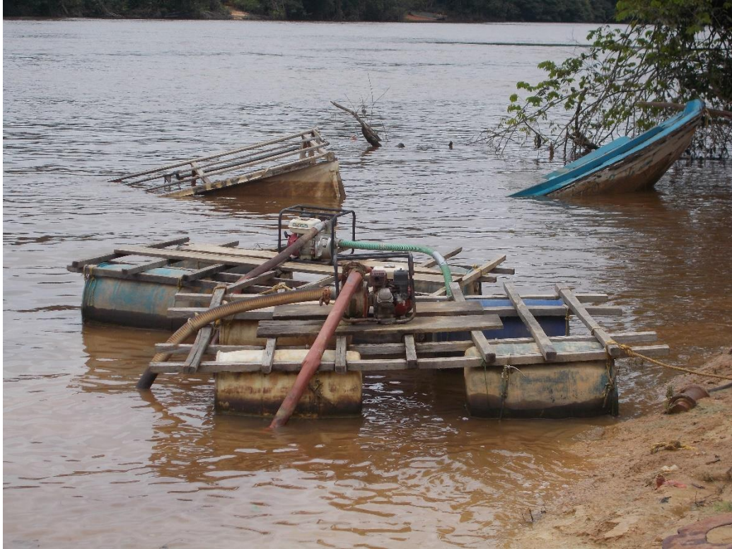
Figure 23: Current practices contributing to oil and grease in waterways in the concession area
