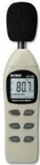
Figure 34: Illustration of Noise Recording device used at SFEP 2/2020
