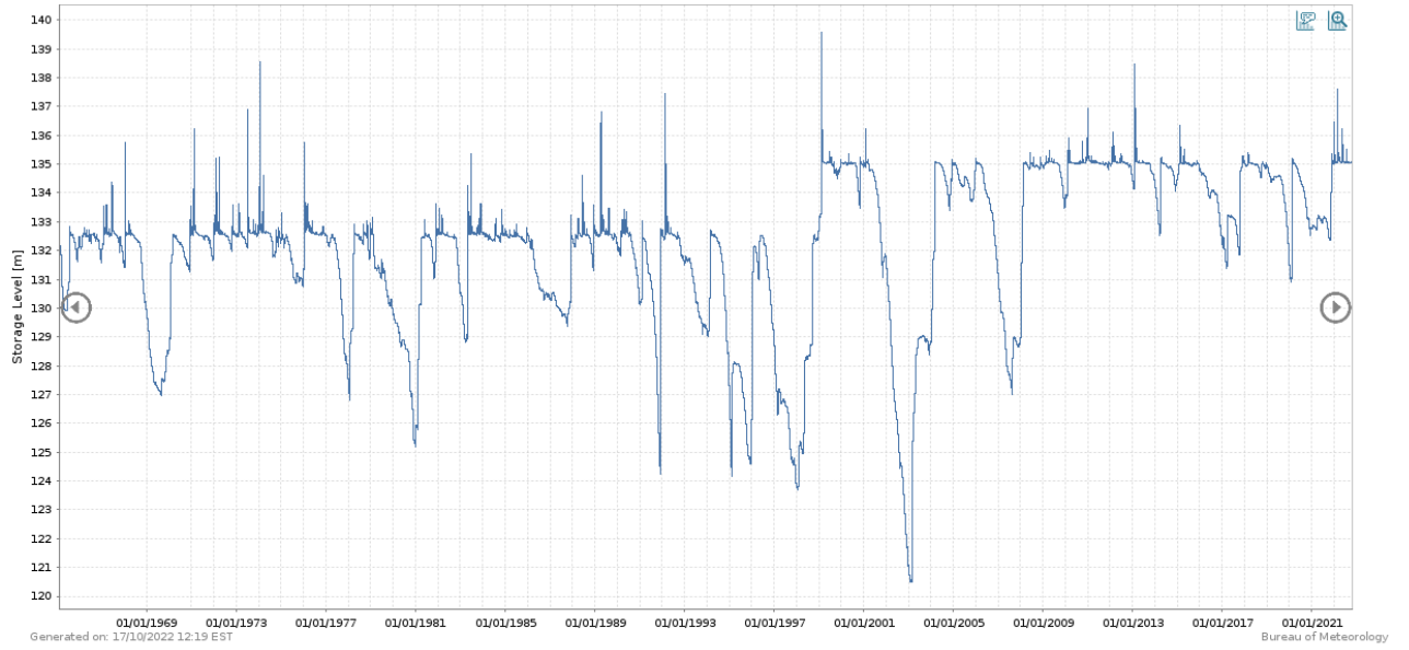
Figure 4-7 Daily mean Borumba Dam headwater storage level statistics from 1965-2022 (138112A).
