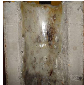
Figure 3. The reinforcement sidewall effect by the EVA hot melt adhesive
