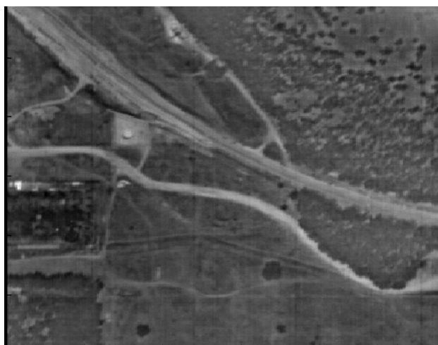
Figure 3. The dataset “field” is a hyper-spectral image of a field taken from an airplane flying 9,500 feet above sea level. The resolution is 1.2 meter/pixel, 286 \times 300 pixels per waveband with 50 wavebands
