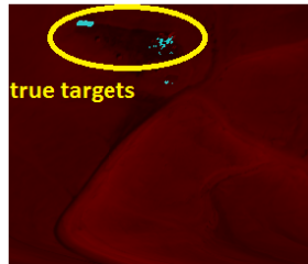
Figure 15. The detected targets by the OSP Ahmad & UI Haq (2011) algorithm are marked on portion of one wavelength from the “desert” image. OSP produces more false-alarm than WDR
