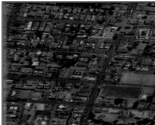
Figure 2. The dataset “city” is a hyper-spectral image of a city taken from an airplane flying 10,000 feet above sea level. The resolution is 1.5 meter/pixel, 294 \times 501 pixels per waveband with 28 wavebands
