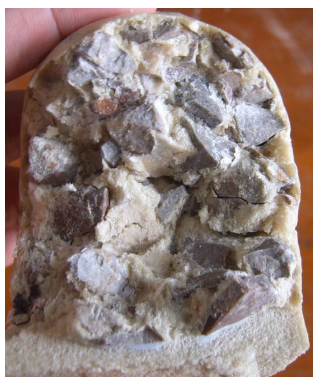
Figure 5. Formed concretion body of polyurethane and water
