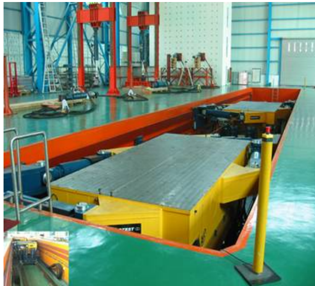
Figure 1. Three-axial shaking table system
