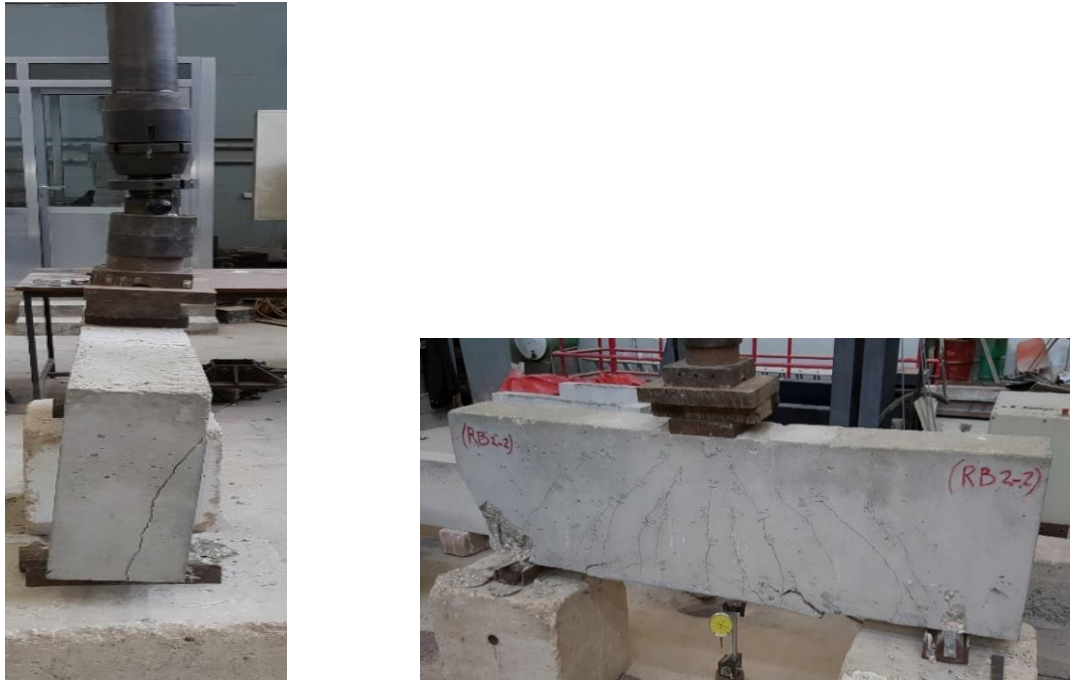
Figure 7. Tilting of Specimens
