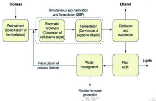
Figure 1: Process flow of biomass to ethanol generation (Source: http://pubs.rsc.org/services/images/RSCpubs.ePlatform.Service.FreeContent.ImageServie.svc/ImageService/Articleimage/2015/RA/c5ra12735a/c5ra12735a-f5\_hi-res.gif)
