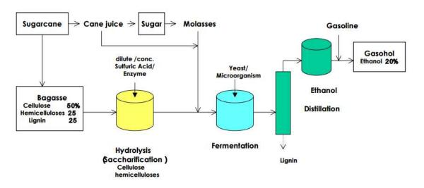
Figure2 : Flow diagram of the ethanol production process (**Source:** http://www.ee-design.net/imgEED/IMGCUT/topics/topics20061214/sugarcane.gif)
