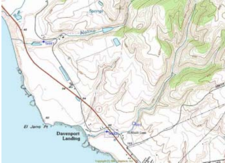
Map 1. Gage 1 is the Molino Creek stream gauge. It is located about 50 feet downstream of the diversion on Molino Creek. Gage 2 is the Ferrari Creek stream gauge. It is located on the west side of Highway 1 and about 1,800 feet downstream of the Coast Dairies diversion.
