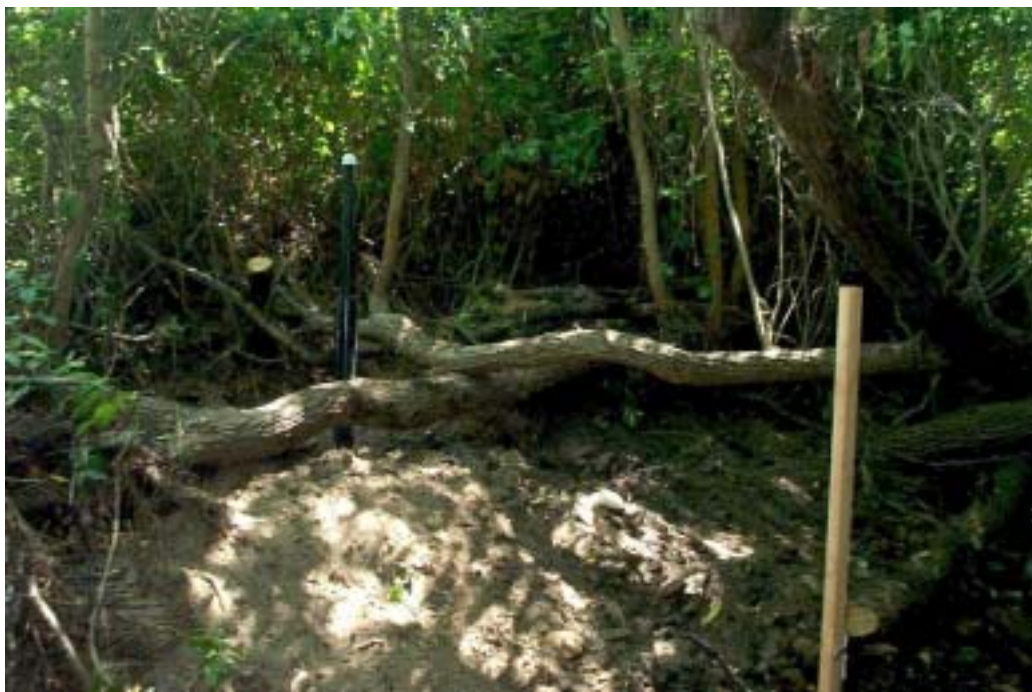
Figure 5. The Liddell Creek staff and stilling well are located about fifty feet downstream of the diversion. The staff plate is located on the side of the 2x4 facing the stilling well. The stilling well is about 12' from the edge of the low flow channel.
