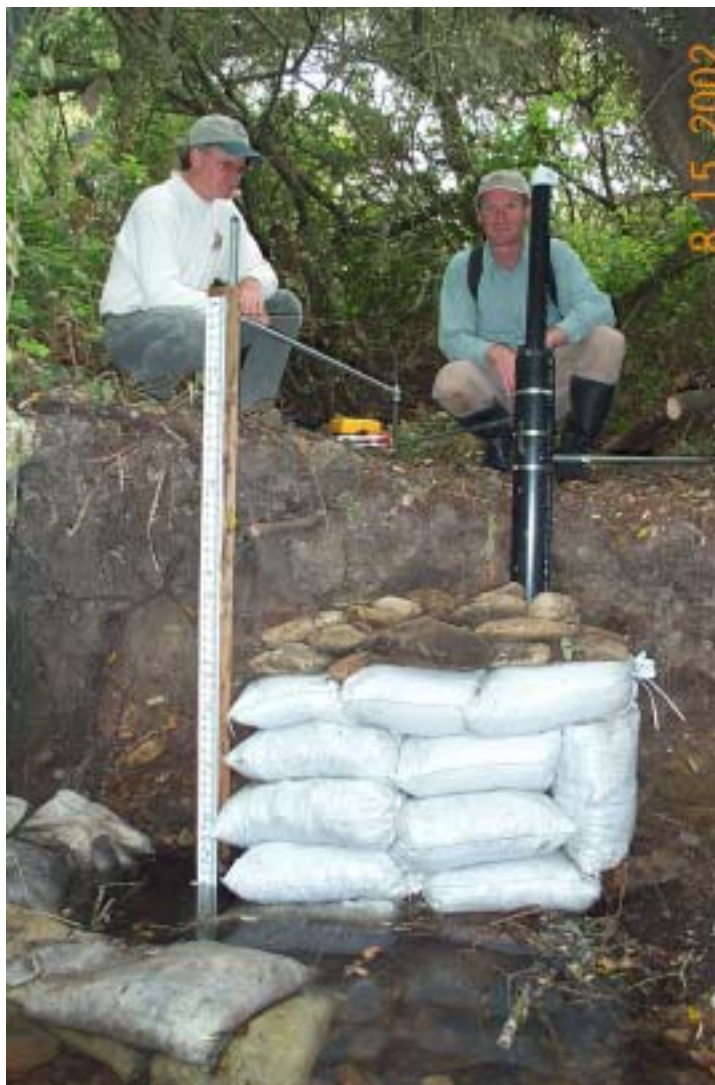
Figure 3. The Molino Creek staff gauge and stilling well for the water level recorder are located about 50 feet downstream of the diversion.
