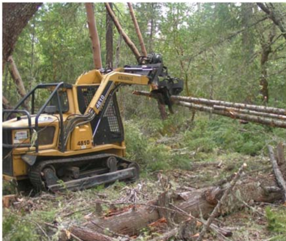
Photo 2-3. Gathering small diameter material with a skidsteer
