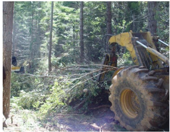
Photo 2-2. Removing biomass from unit in whole tree form
