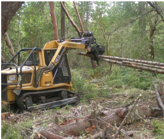
Photo 2-3. Gathering small diameter material with a skidsteer
