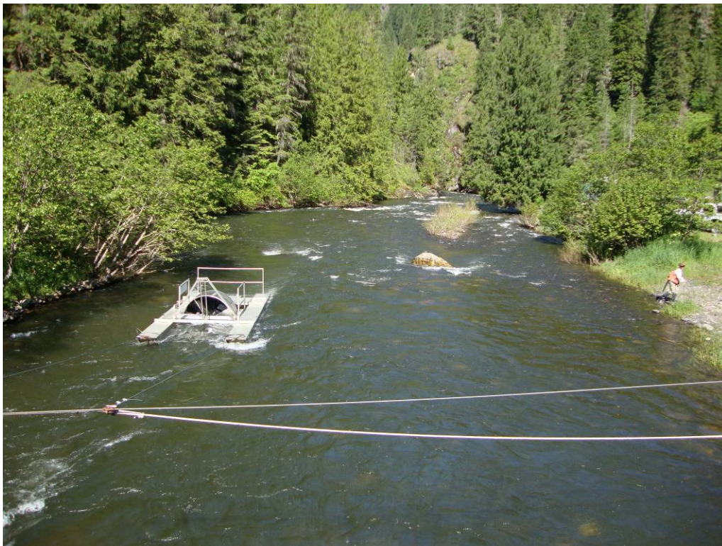
Photo 8. Existing NPT screw trap, showing overhead cable system, June 2011.
