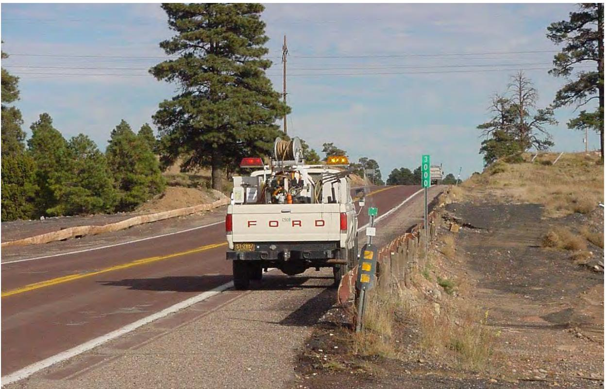
**Photo 2. 4x4 3/4-ton truck with high boom sprayer.**
