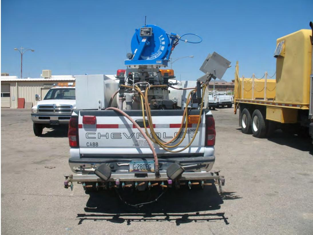
Photo 3. 4x4 3/4-ton truck with low boom sprayer.
