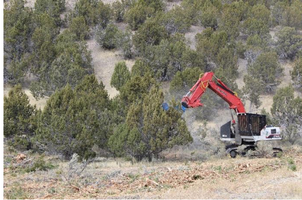
Curlew juniper mastication in progress
