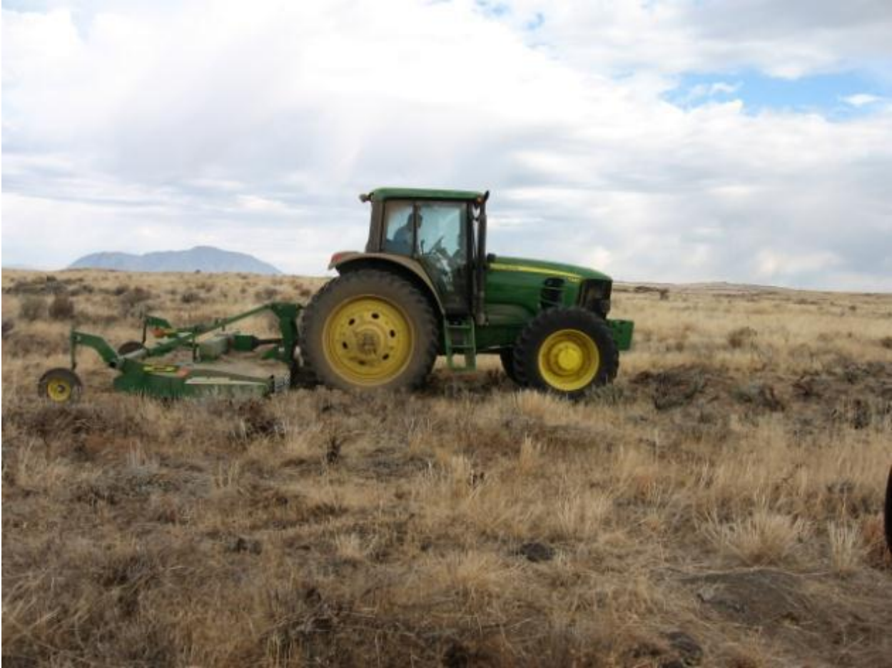
Figure K-25. Rubber-wheeled tractor and roto-mower establishing a fuel break on the Idaho Falls District.
