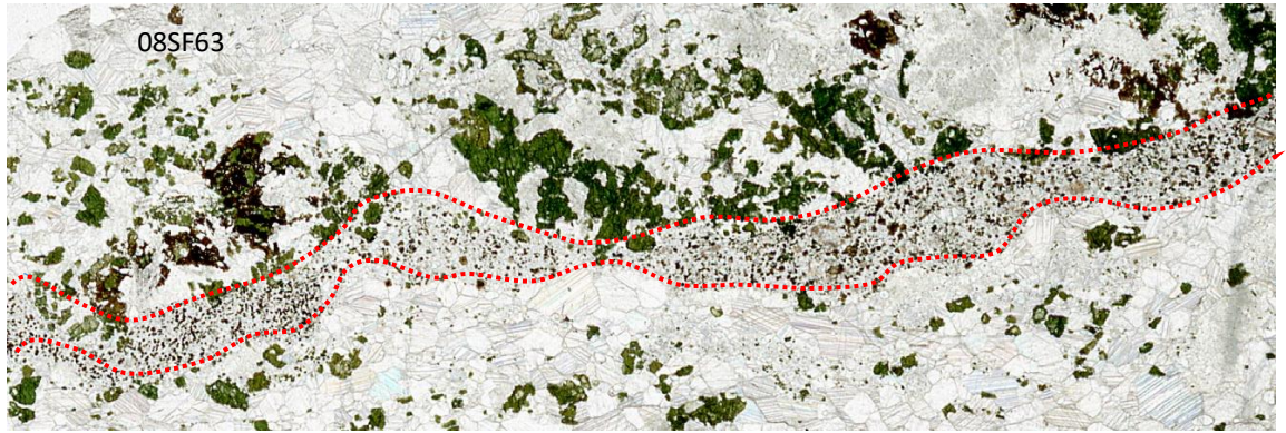
Fig.4.22 Photomicrograph of 08SF63 (FOV 3cm) displaying in upper part calcite-apatite-feldspar (gray), clinopyroxene (green)-rich area separated by fine-grained garnet-titanite from the lower part which contains calcite with minor pyroxene.
