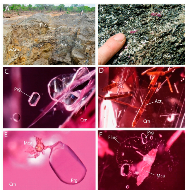
Figure 33. The Mozambican ruby deposits. (A) Ruby-bearing amphibolite (Am) at the M’sawize deposit, Niassa Province, 2009. The weathered amphibolite (wAm) is crosscut by whitish plagioclase veins (Plv); (B) the Maninge Nice deposit, Concession Gemfields, Montepuez, 2012. The ruby (Crn) is surrounded by a plagioclase corona (Pl, anorthite) in a weathered amphibolite (wAm); (C) euhedral pargasite (Prg) in ruby. Field of view 1.5 mm; (D) inclusions of actinolite (Act) in ruby. Field of view 2.5 mm; (E) crystal of pargasite associated with mica (Mca) in ruby. Field of view 1.1 mm; (F) a melted mica (Mca) surrounded by a halo of fluid inclusions (Flinc) arranged in a “butterfly wing” indicative of decrepitation and recrystallization phenomena. The pargasite is euhedral and devoid of deformation. Field of view 1.7 mm. Photos A and B: Vincent Pardieu © GIA. Photos C to F: Jonathan Muyal © GIA.
