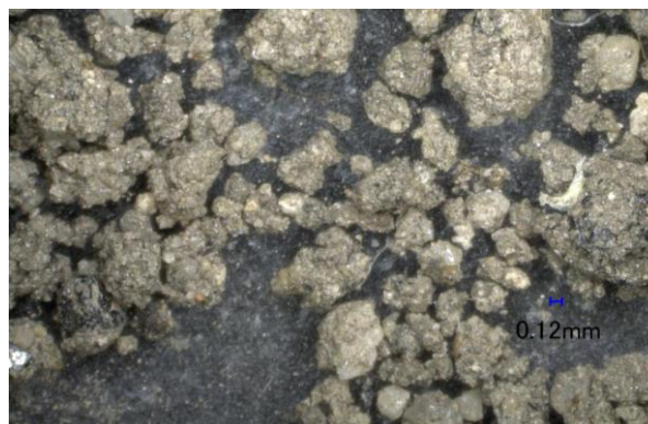
Fig 97: Microscopy image of soil particles used in the burial experiment. Scale = 0.12mm, x26 magnification
