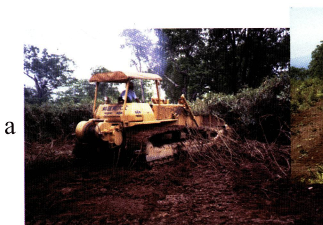
Photo. 7. We employ a bulldozer with upward-warped rakes (a) for site preparation to partly eliminate dwarf bamboo and litter with microorganisms (b).
