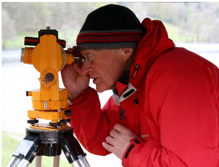
Plate 2: A Disto mounted on the telescope of a theodolite
