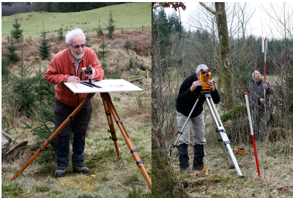
Plate 3: Surveying using a plane table and a theodolite and Disto
