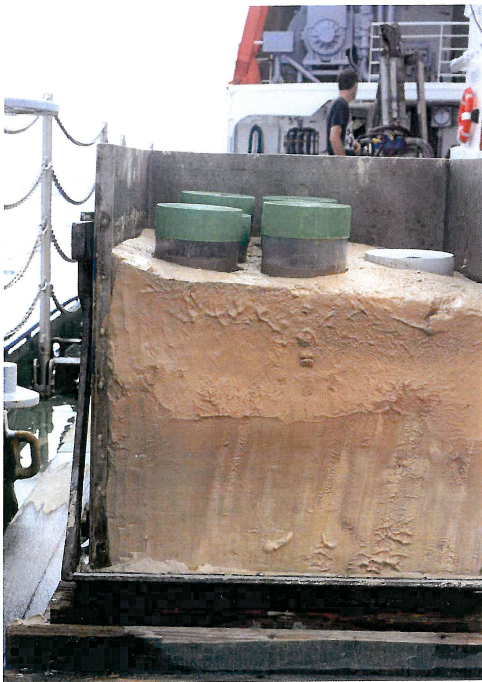
Figure 2.4: Boxcore on deck with subcore tubes inserted Subcore tubes were inserted and pushed vertically into the sediment before the side of the box was removed. Tube diameter is 11.4cm. Box has a 50cm x 50cm footprint and is 60cm high.
