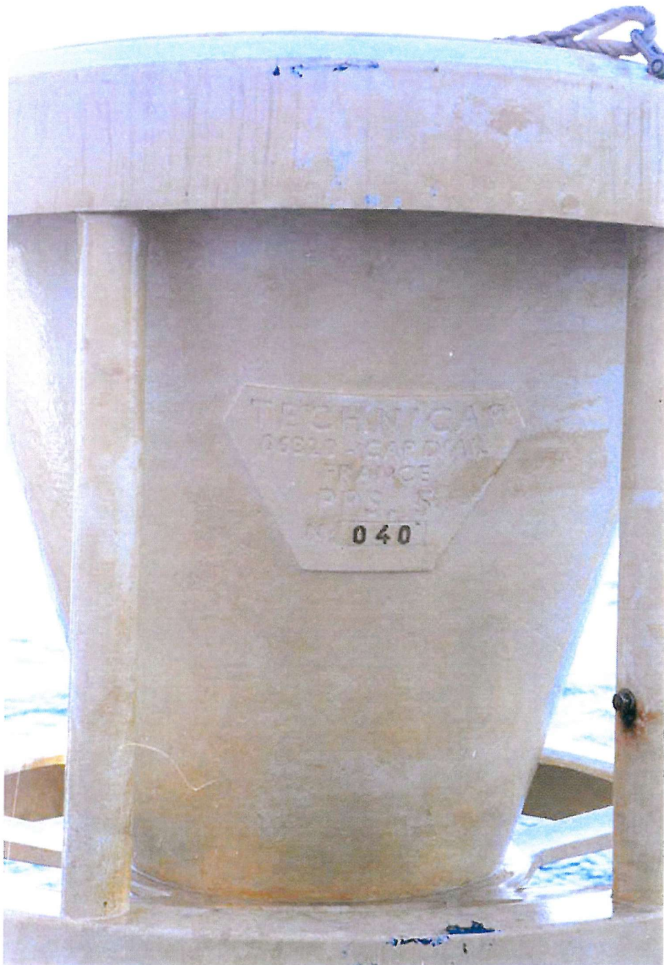
Figure 2.6: Sediment trap coated in orange-coloured sediment. This trap was one of the pair on the near-field mooring, located 500m from the vent site. The traps on the distal moorings did not have this coloured coating of sediment on recovery.
