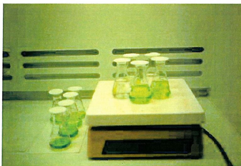
Figure 2.12: Dissolution of NiS beads for Os and PGE analysis
