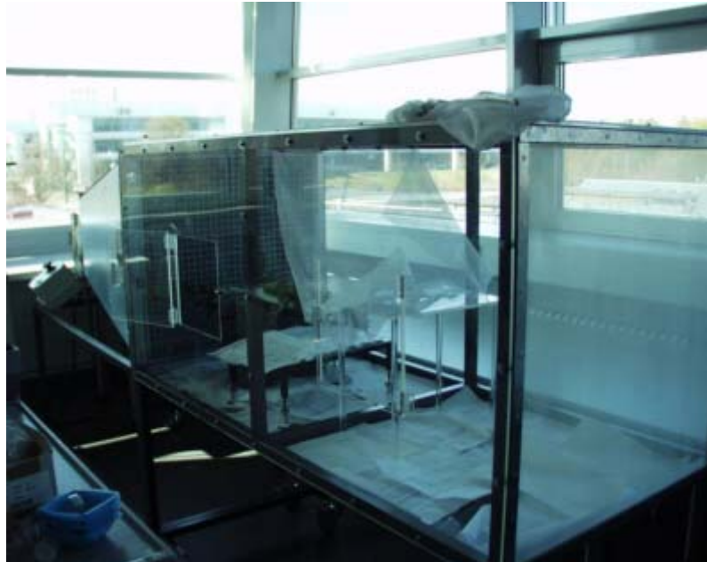
Fig. 5.2: View of the wind tunnel, in which experiments analysing the usage of different senses were conducted. The motor with the charcoal filters is on the left, on the right the flight chamber. In the rear the large windows are visible.
