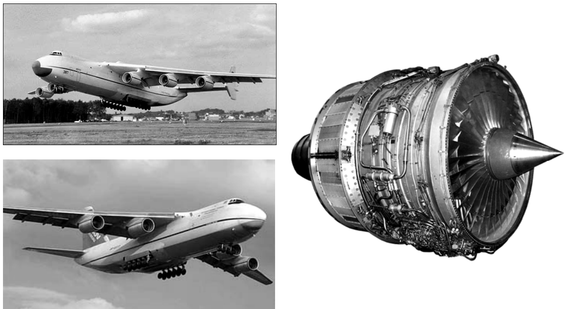
Fig. 3.1. The Д-18 engines power “Ruslan” and “Mrij” aircraft
