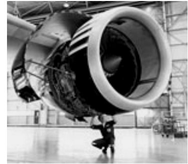
Fig. 3.2. RB211-535E4 engines power the Boeing-757 and Tupolev Tu-204 aircraft
