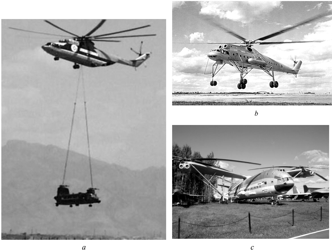
a b c Fig. 1.20. Helicopters: a — Mil Mi-26 recovering an American CH-47 Chinook helicopter; b — Mil Mi-10; c — Mil V-12, largest helicopter in the world
