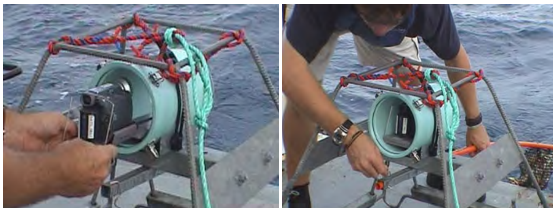
Figure 2-20: Applying camera and bait arm to BRUVS before deployment. Note ballast on frame and 8 mm hauling rope.
