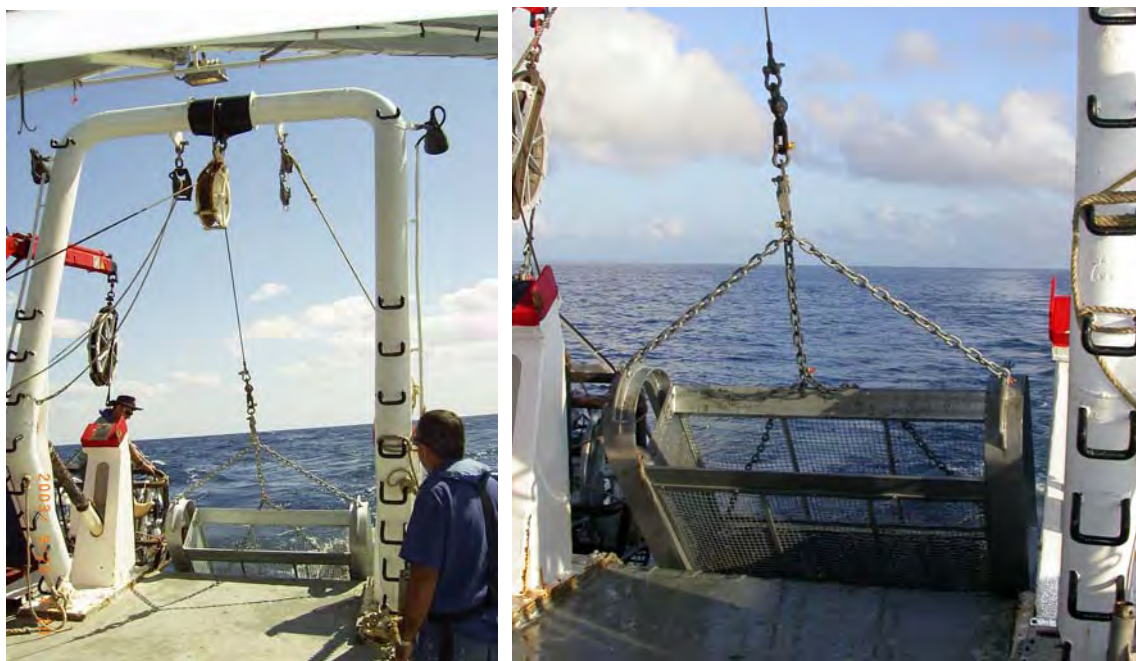
Figure 2-21: The epibenthic sled being deployed through the A-frame for a 200 m tow along the seabed; note the weak link at the top of the bridle and retrieve chain leading to the rear of the sled.
