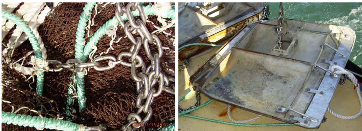
Figure 2-24: Drop chain links and trawl boards.
