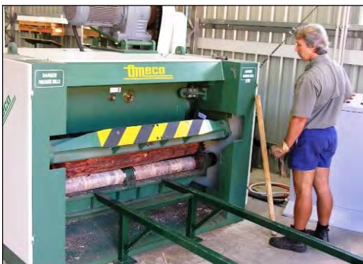
Plate 1.4. Processing a peeling billet in the 'Omeco' spindleless lathe – Eric Littee
