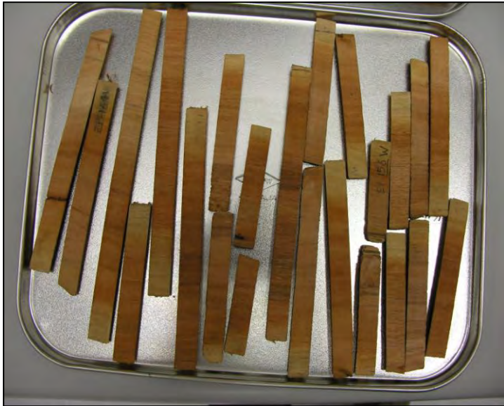
Plate 1.13. Core samples of E. pellita after seven days exposure to ultraviolet light
