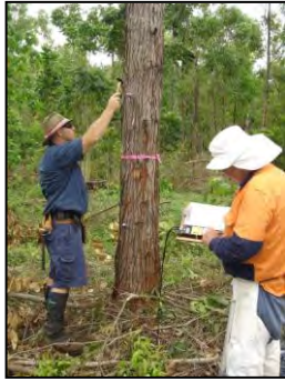
Plate 1.1. Using a Fakopp Microsecond Timer – Martin Davies and Terry Copley
