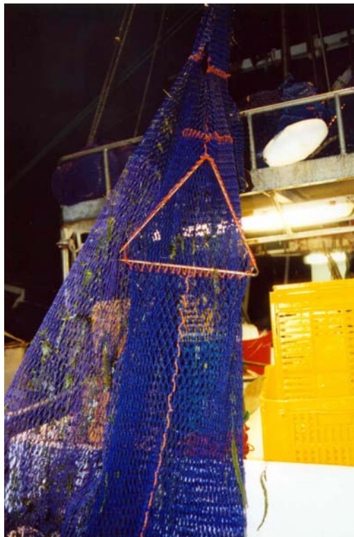
Figure 8.3.1. The fisheye BRD as used by Mr Reg Saunders on the Lewis Venture (FPPX). The effects of this device on prawn, whiting and bycatch catch rates were evaluated.
