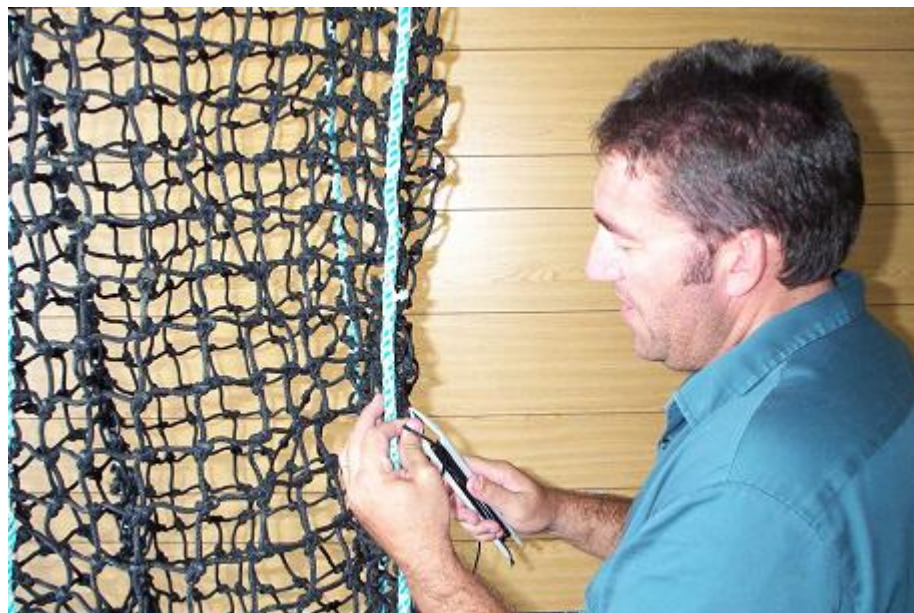
Figure 7.3.2. The square mesh codend BRD under construction. Note the large open squares (50 mm x 50 mm). The 12 mm polyethylene rope was selvedged along the sides to take the weight of the bycatch and prevent distortion of the mesh.
