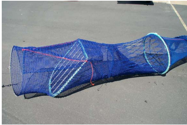
Figure 5.3.2. The radial escape section BRD and TED after construction. Note the large escape meshes are restricted to the upper half of the codend circumference.
