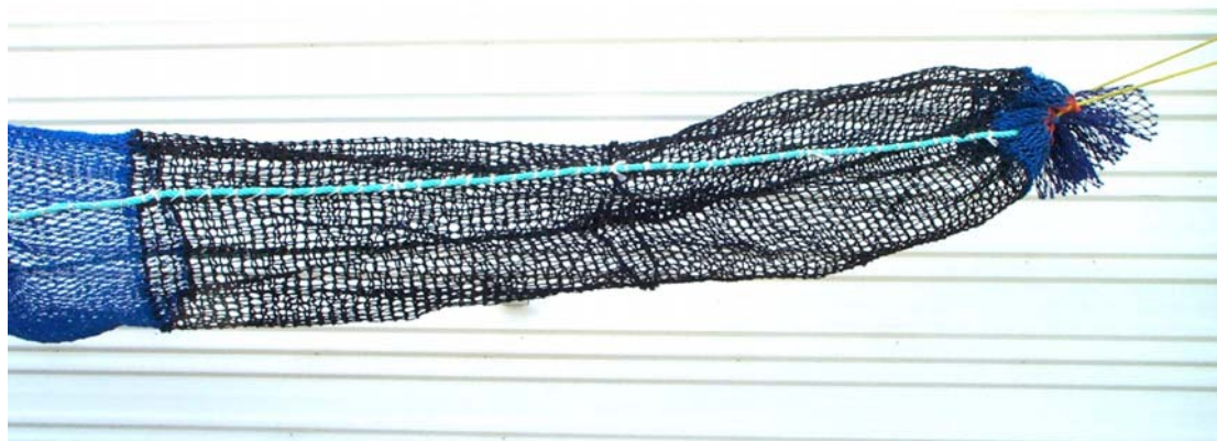
Figure 9.3.2. The square mesh codend BRD that was evaluated during the deepwater eastern king prawn charter was constructed from 17/8 inch black braided polyethylene. The square mesh section was 66 bars round and 76 bars long. Note that a short section of diamond mesh was added to the aft edge of the square mesh so that the drawstrings could be attached in the normal manner. The rope was added to reduce knot slippage.
