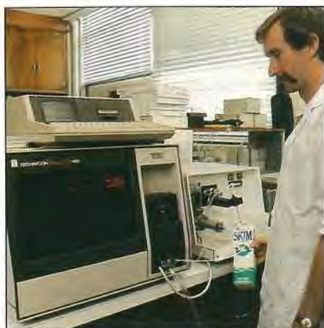
Plate 2. An Infra-red analyser used for the simultaneous determination of fat, protein and lactose in dairy products.
